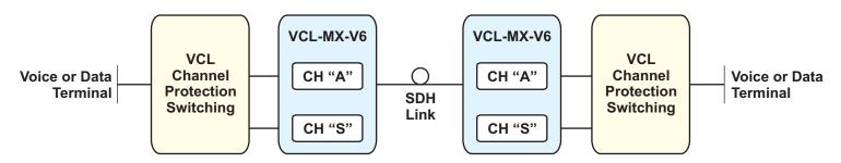
CH "A": Active Channel (Voice or Data) / CH "S": Standby Channel (Voice or Data)
