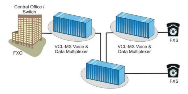
FXO/JNC 2 wire exchange loop interface card FXS/SLC 2 wire subscriber loop interface card
