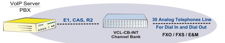
The cable plant of most telecom service providers is not designed to deliver E1 services to customers in most parts of the world. The VoIP Gateway / Switch / Server / PBX with an E1 interface, thus, in such cases can only be accessed through dial-up, 2 wire analog lines, the only available link for connecting the Exchange (Central Office) to the Corporate PBX Networks and VoIP (Voice over IP) Gateways.
