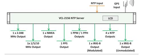
The VCL-2156 is equipped with a highly accurate, low-noise OCXO to provide a high stability, ITU-T G.812, Type II, III compliant holdover clock with better than 12 $\mu$ s accuracy over a 24 hour (5 milliseconds per year) period in the event of unavailability of the GPS / GNSS signal, or GPS / GNSS antenna failure, or a temporary loss of reception in a totally isolated network without any external reference.
