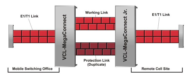
During normal operation, MegaConnect sends duplicate traffic across both the working and dedicated protection E1/T1 facilities while continuously maintaining the performance of both links to determine which link shall be utilized.
