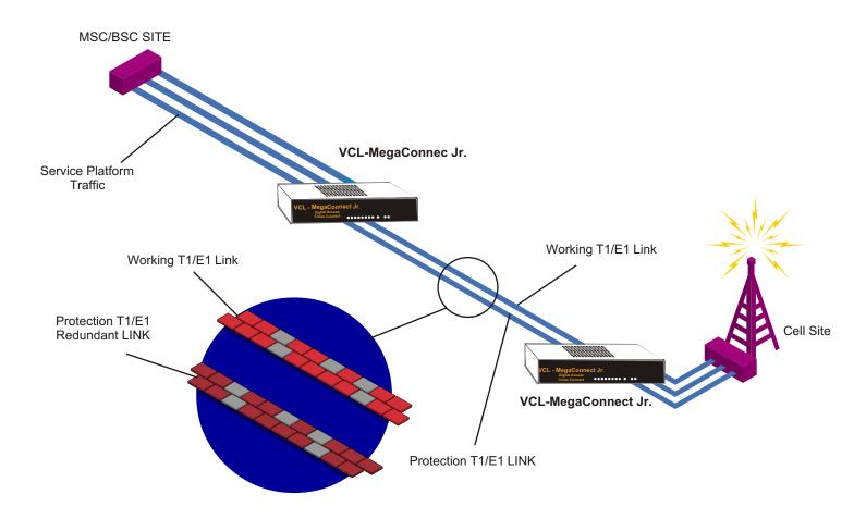
These ensure that mission critical voice, data, control and management traffic are properly supported and maintained even during T1/E1 backhaul facility outages. When the working link fails, the protection link becomes active.
