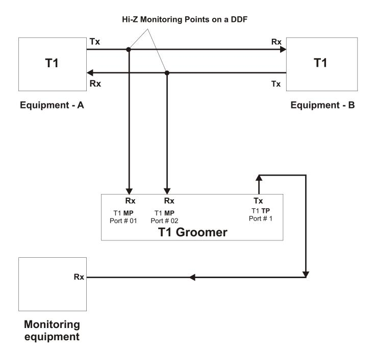
Where TP is testing T1 Point and MP is Monitoring T1 Point.
