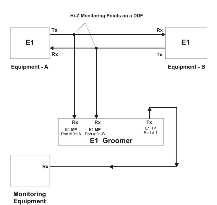
Where TP is Testing E1 Point and MP is Monitoring E1 Point.
