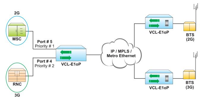
**Notes:** Flow Control feature allows the user to regulate the Ethernet traffic flow to minimize link to minimize packet loss due to data bursts.
