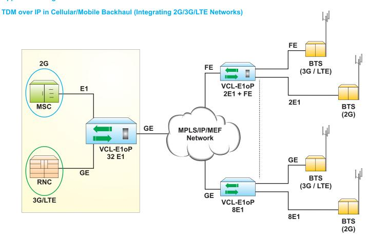
TDM over IP for 2G/3G/LTE - Typical Application in a redundant Wireless Network (1+1 Link Redundancy)
