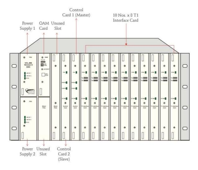
The equipment provides a wide choice of access ports for connecting to and executing management and configuration commands through its OAM Card.
