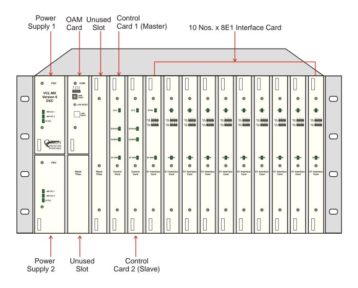
The equipment provides a wide choice of access ports for connecting to and executing management and configuration commands through its OAM Card.
