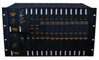
time-slot (DS-0) cross-connect fabric for up to 80 E1 ports. This product offers 1+1 -48V DC Power Supply Redundancy, 1+1 Control Card and Processor Redundancy, 1+1 Cross-Connect (TSI) Redundancy, 1+1 Timing (Synchronization Clock Circuitry) Redundancy. This DXC offers "user selectable" clock / timing synchronization priority. The Dual Power Inputs allow the equipment to be powered from two separate power sources. AC input external adapter is an optional for AC mains operation.
