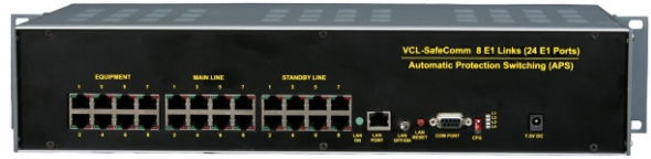
VCL-SafeComm, 8 E1 Links (24 E1 Ports) 1+1 Automatic Protection Switching (APS)
