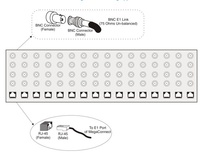
VCL 75 Ohms Patch Panel with Hi-Z Monitoring Port is used for E1 Monitoring Application.
